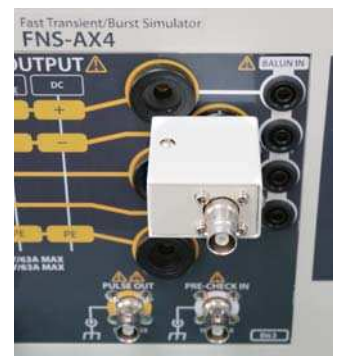
02-00152A adapter mounted onto L2(N-) port of EUT LINE OUTPUT
